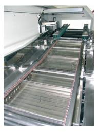
installed in the fluxer and preheat area, is provided with Viton O-rings to ensure a save transportation of the assemblies to be processed. In the soldering area, the assemblies are taken over by teflon coated fingers.
