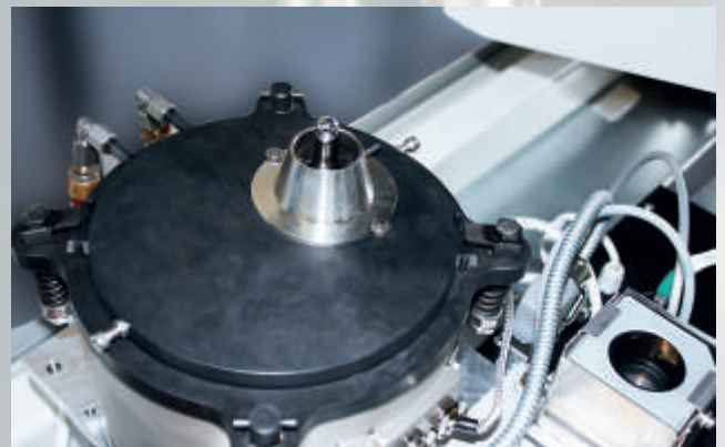
electro-magnetic soldering unit: miniwave or dip soldering processes
