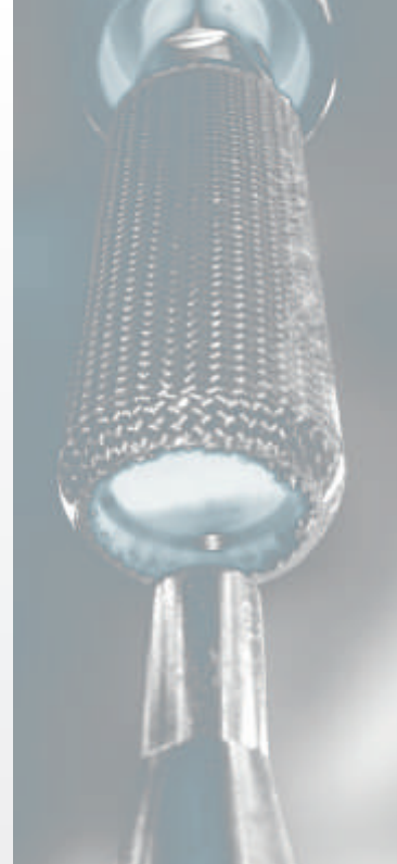
automatic ultrasonic solder nozzle cleaning patented by SEHO
